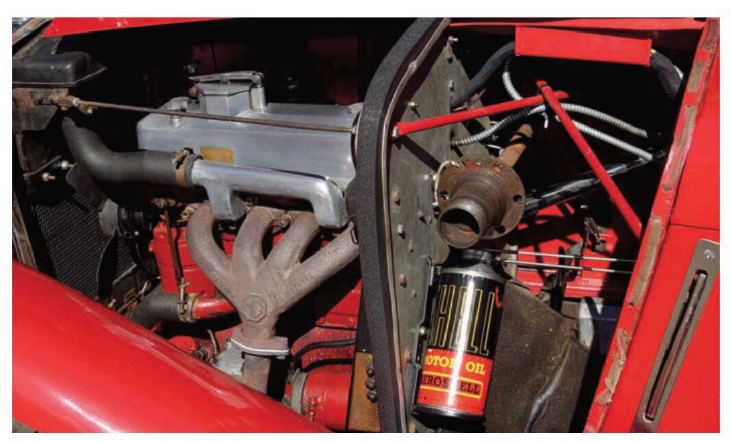
New crossflow motor for P-Type was still 847cc, but made 36bhp@5500rpm.
