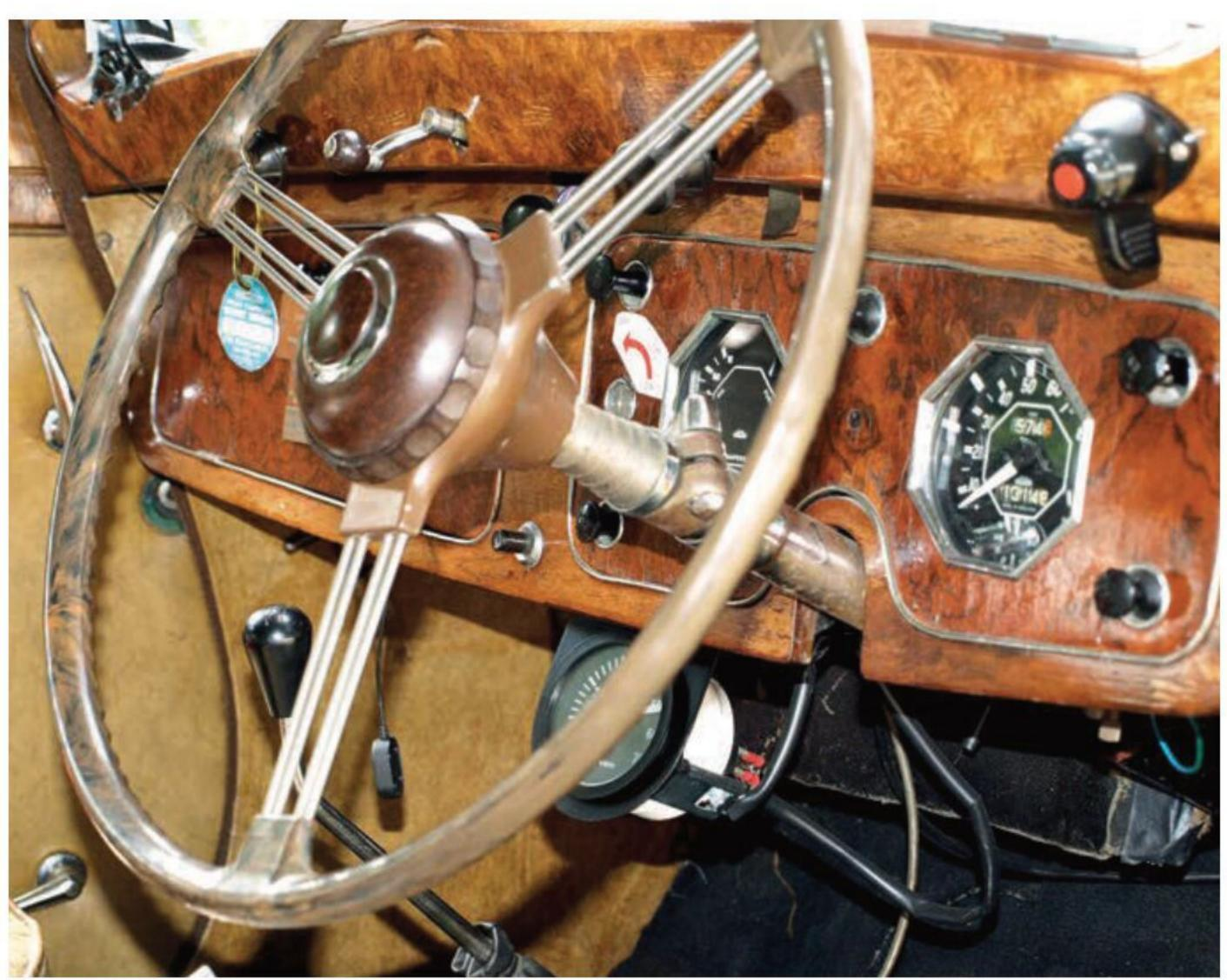
Steering wheel and dashboard instruments remain original; the only addition is an electric tachometer fitted beneath.
