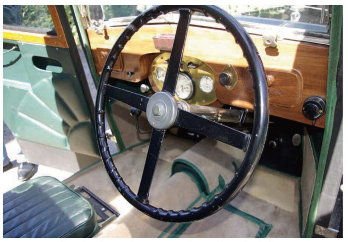
Gauges are gathered in a brass plate, positioned centrally on the dash.
