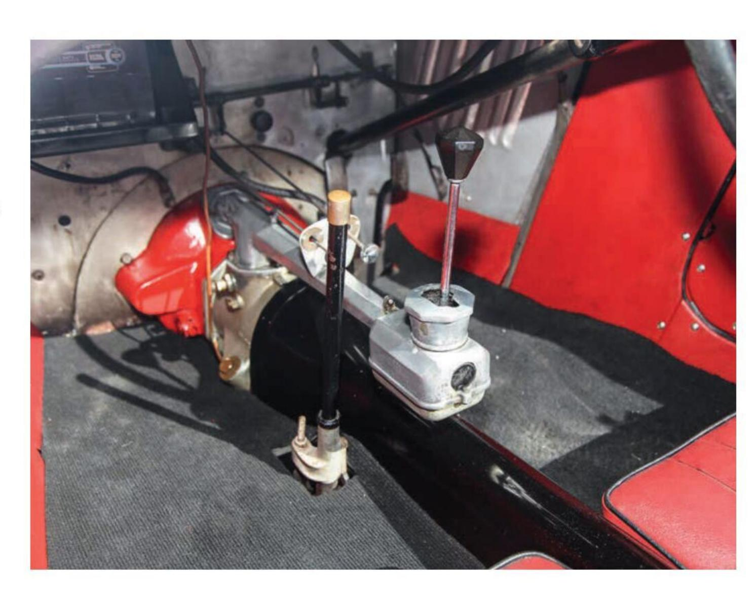
pressed. Changing gear in the J2 can take a little bit of practice, not only ensuring the driver becomes proficient in double de-clutching because of the absence of any synchros, but also due to the fact
